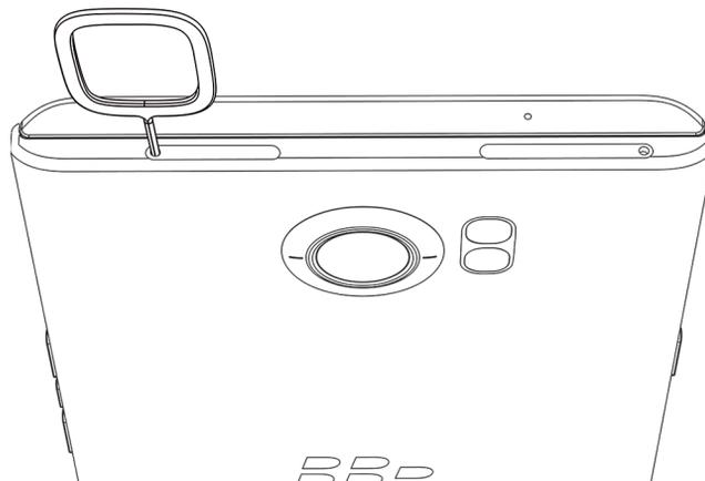
3. Pull out the tray completely and set it on a flat surface.
