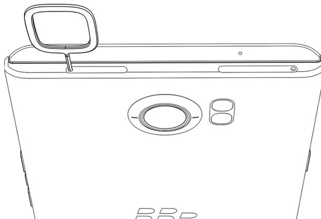
3. Pull out the tray completely and remove the media card.
