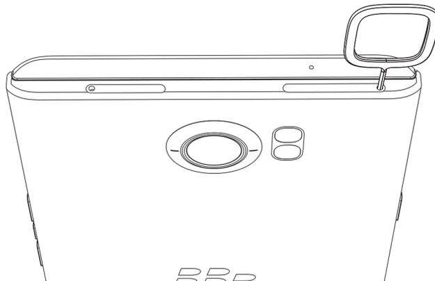
3. Pull out the tray completely and set it on a flat surface.
