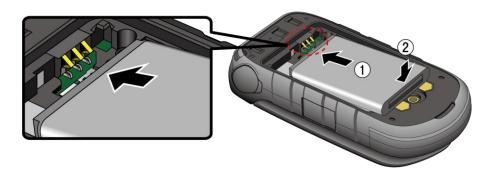
4. Replace the battery cover, making sure all the tabs are secure and there are no gaps around the cover.
