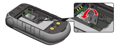
3. Slide the microSD card into the slot with the gold contacts facing down. Gently push the card in until it snaps into place.
