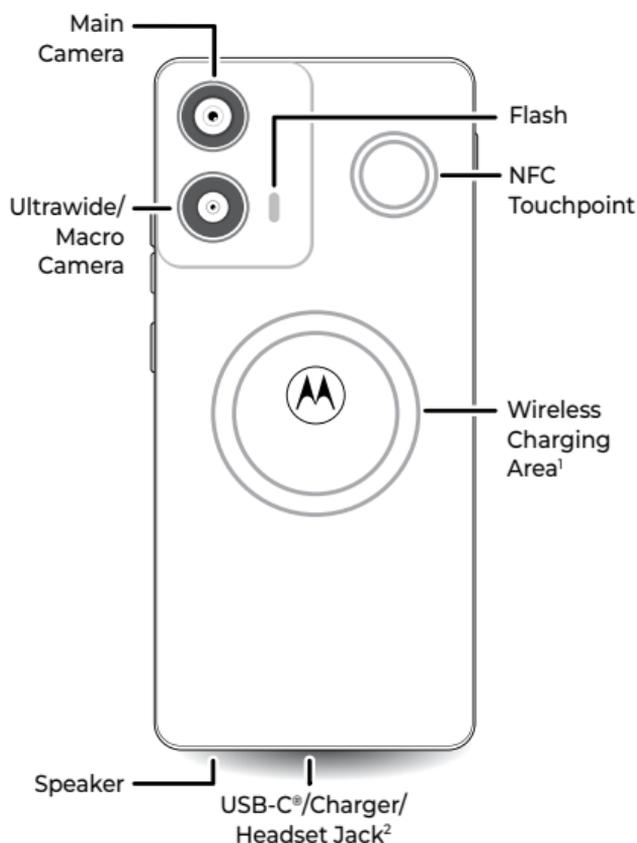
**<sup>1</sup>Wireless charging:** Charge your phone using a Qi-certified wireless charger (sold separately). To achieve the best charging performance, align the wireless charging area of your phone with the wireless charger, or place your phone in the location recommended by the charger manufacturer. See [Check your battery charge level](#).
