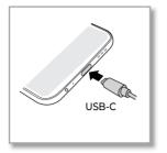
Charge your phone using a compatible Motorola charger (may be sold separately). Use of other chargers is not recommended. Insert the charging cable into the charging port (see **First look** for port location). Plug the other end into a power receptacle.
