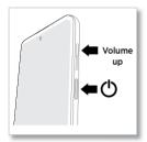
**Tip:** You can adjust settings, if you want to only press and hold the Power button (instead of the Power and Volume Up buttons) to turn off the phone. See **Gestures**.
