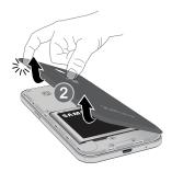
**Warning**: Do not bend or twist the back cover excessively. Doing so may damage the cover.
