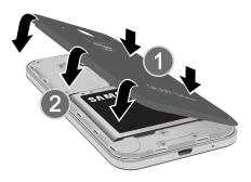
3. Press along the edge of the back cover until you have a secure seal.
